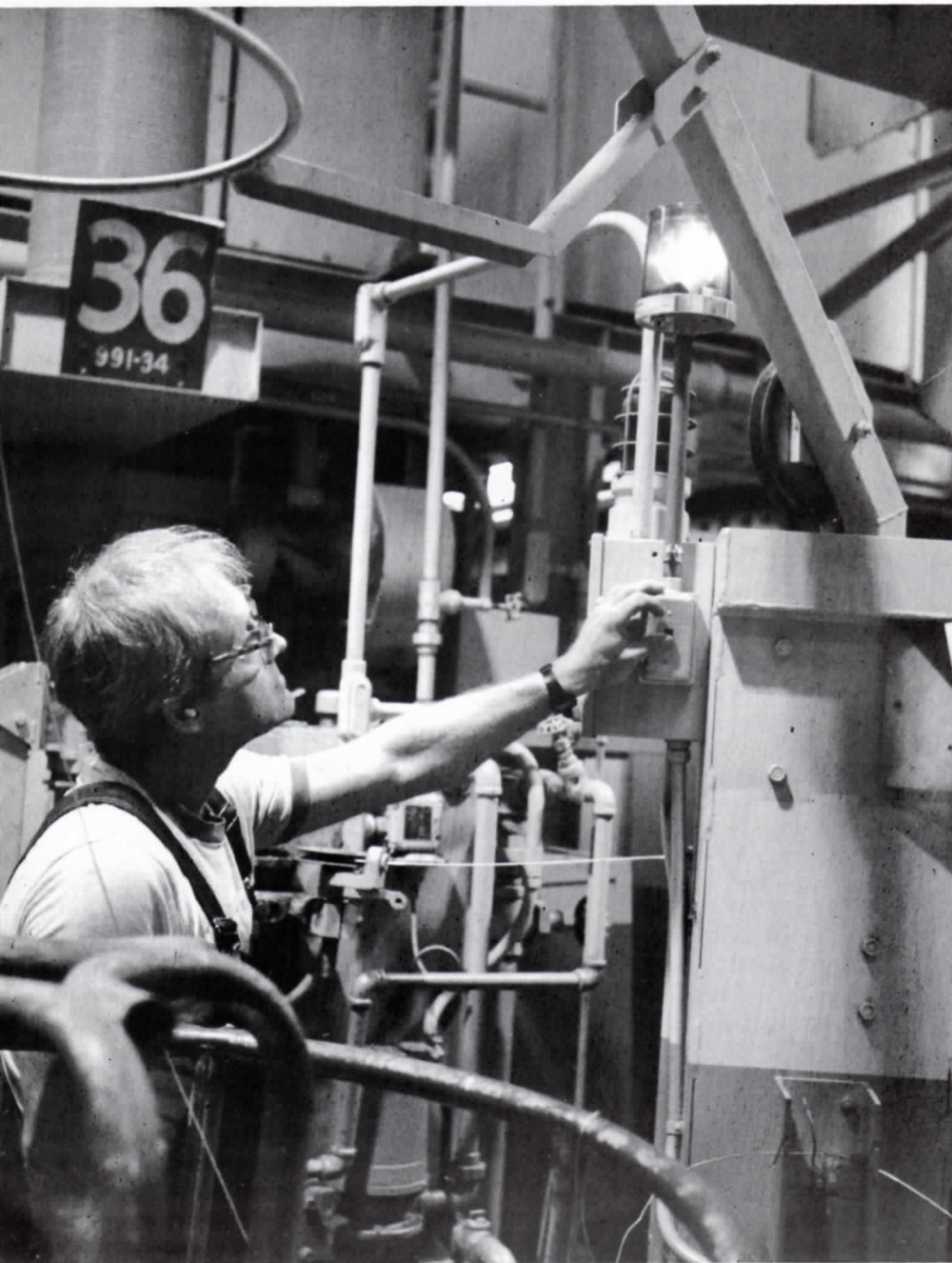
BLUE LIGHT SPECIAL . . . When insulating line operator Steven Prerost needs an ink room attendant to service his line’s color coder, he just turns on a newly installed blue flashing light.
