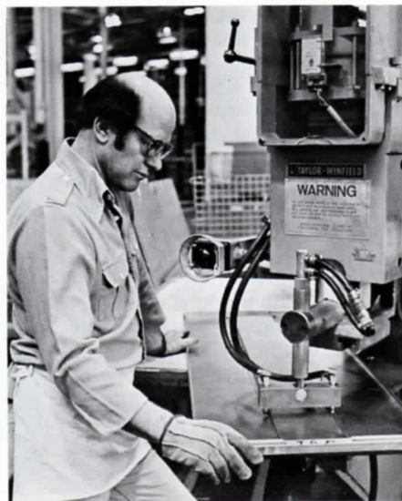
FIRST THINGS FIRST . . . Machine operator Frank Schleimer of Dept. 437 welds 3A panels before they are to be painted.
