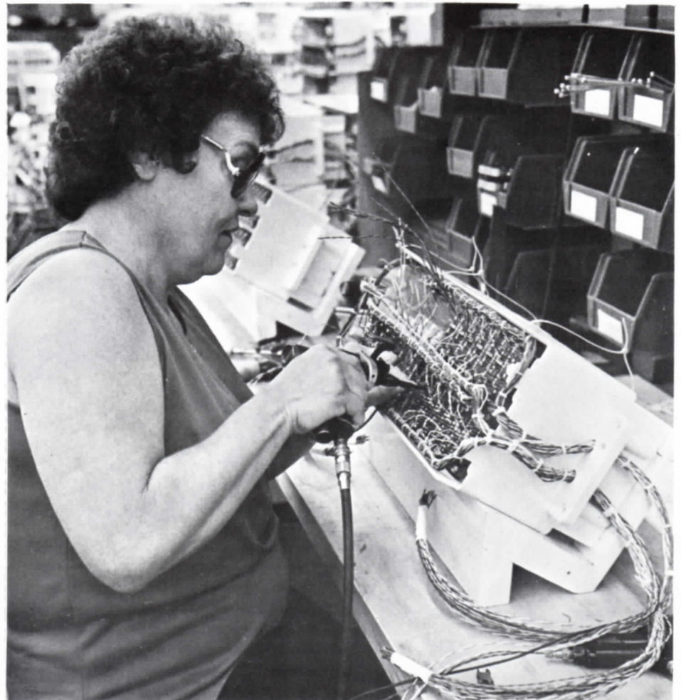
SPAGHETTI DUTY . . . One of Betty Drews's duties as a wirer in Dept. 439 is to wire repeater shelves used in the 41-type cabinet.
