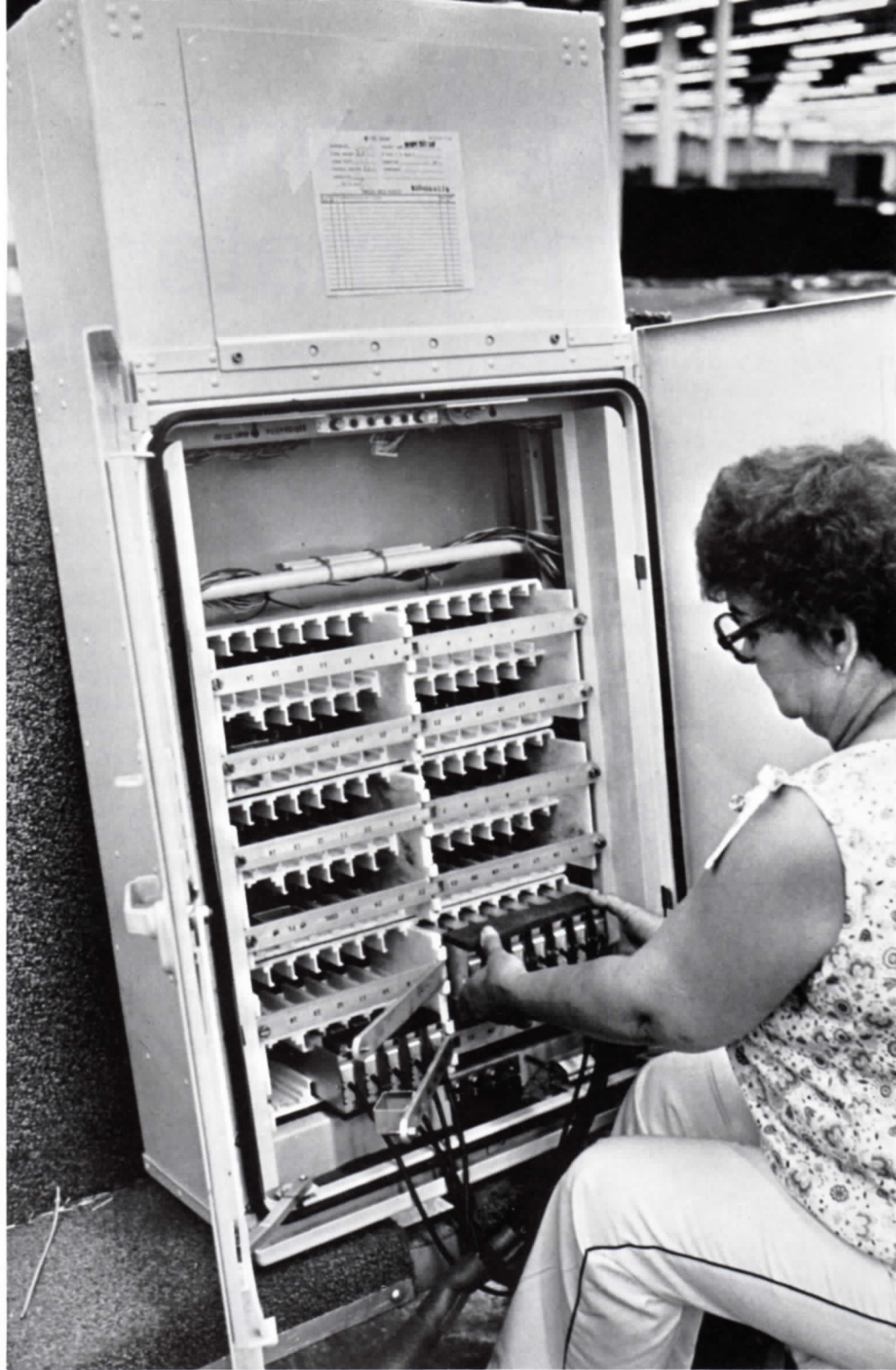
CHECK IT OUT . . . Ida Flott of Dept. 439 tests repeater shelves in a new 841 repeater case. The case is upside down to make assembly easier.
