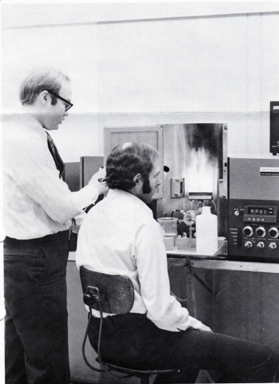
The atomic absorption spectrophotometer has an important function in determining metal content in water. Jerry, left, and Louis Canal, assistant chemist, run a sample test.
