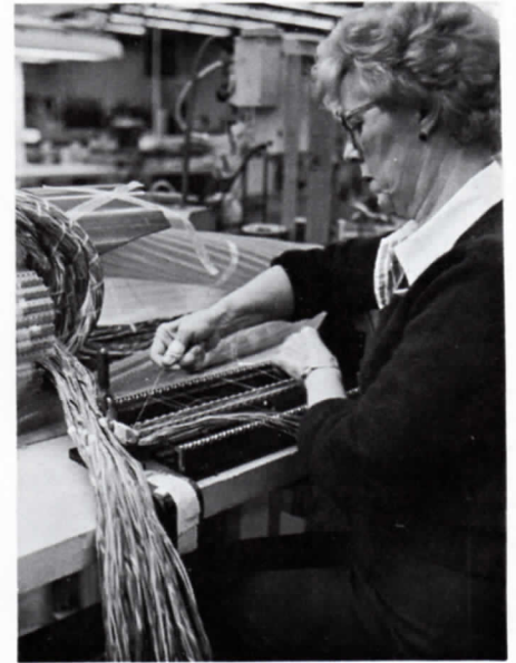
LOTS A WIRE . . . Wireman Lorraine Haverman of Dept. 444 had her hands full wiring 4200-pair cable attached to a special-ordered load coil case.
