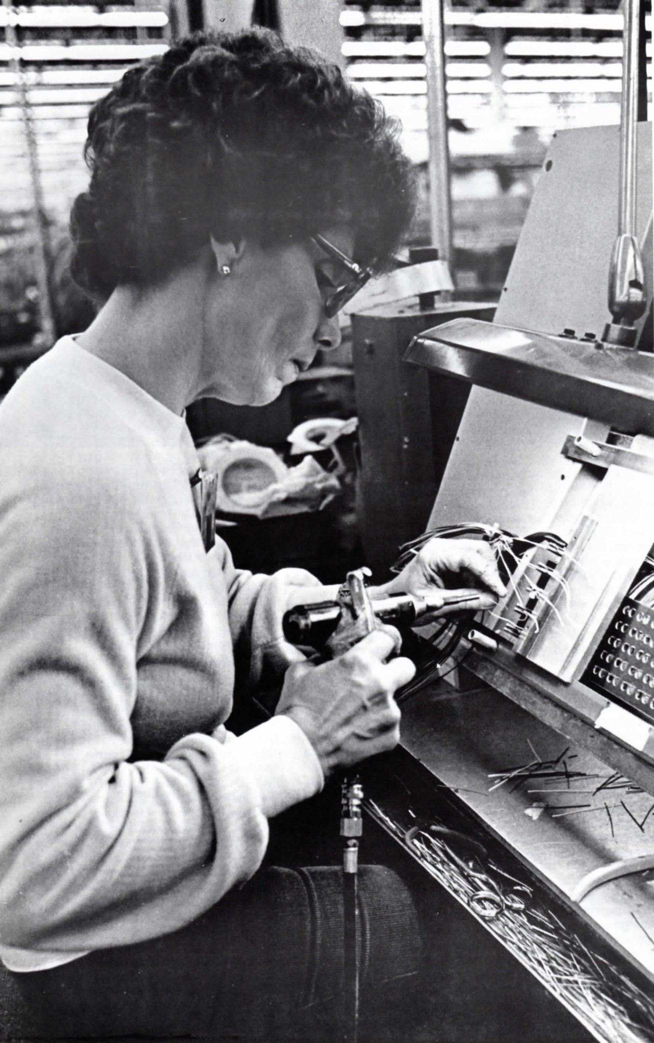
PRECISION COUNTS . . . Wirer Mary Purcell of Dept. 442 must know what color-coded wires go where when she works on 189 building entrance protectors. The wiring gun she uses will be replaced with a new one featuring a built-in wire stripper.
