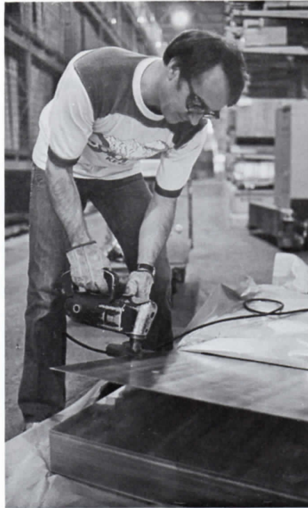
CAREFUL HANDLING ... Raw materials inspector Mike Miller uses saws and a small mill to take samples of steel sheets. Careful attention to safety ensures he won't be cut in the process.
