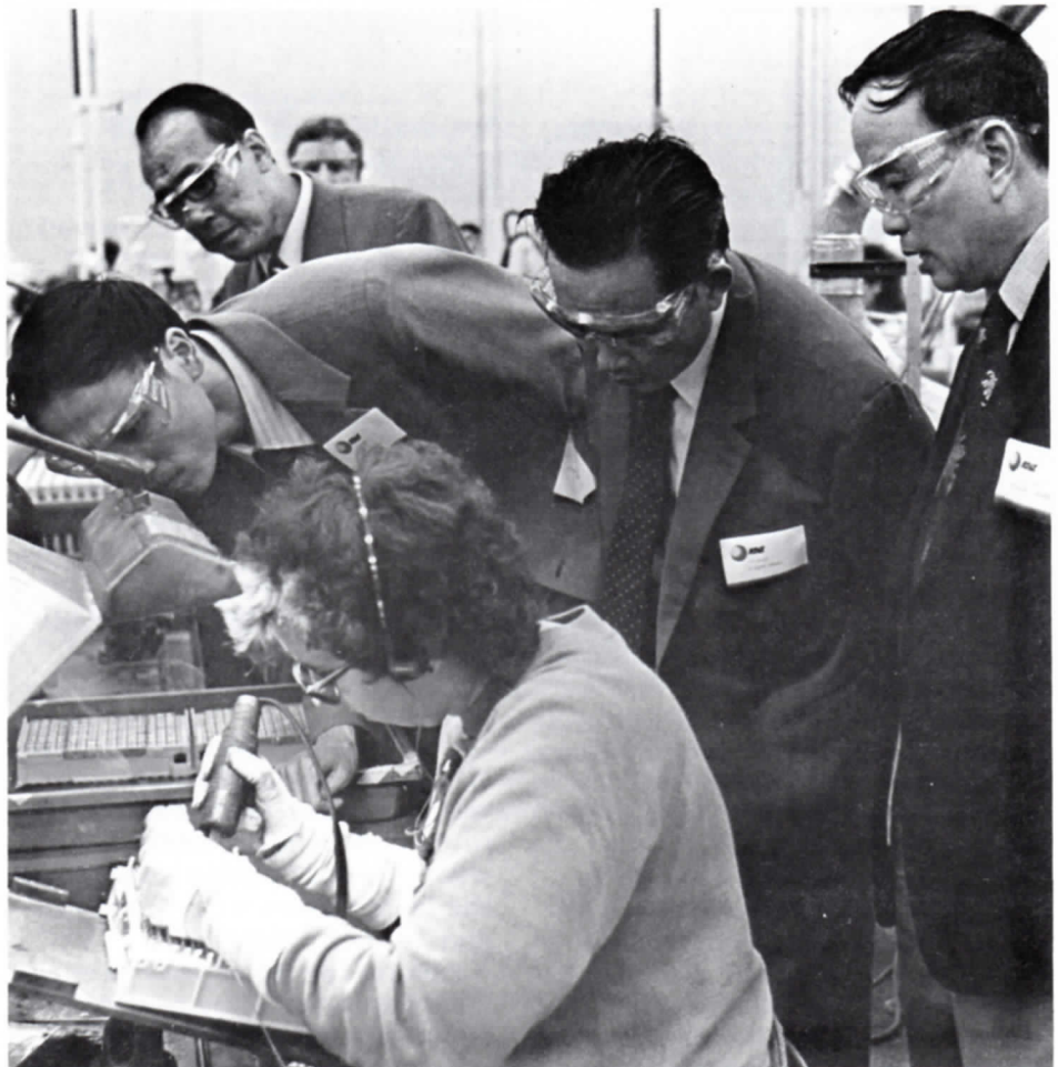
WATCHING CLOSELY . . . Lana Baxter of Dept. 442 had the undivided attention of the visitors as she soldered a 128 central office connector panel.
