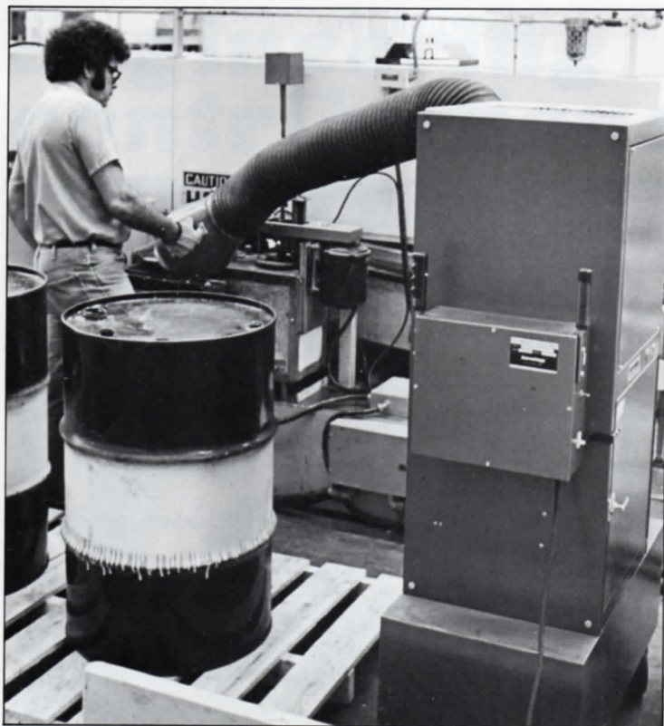
A new electrostatic precipitator exhaust helps Dick Hinkle, 441, when removing solder dross from the circuit pack wave soldering machine.
