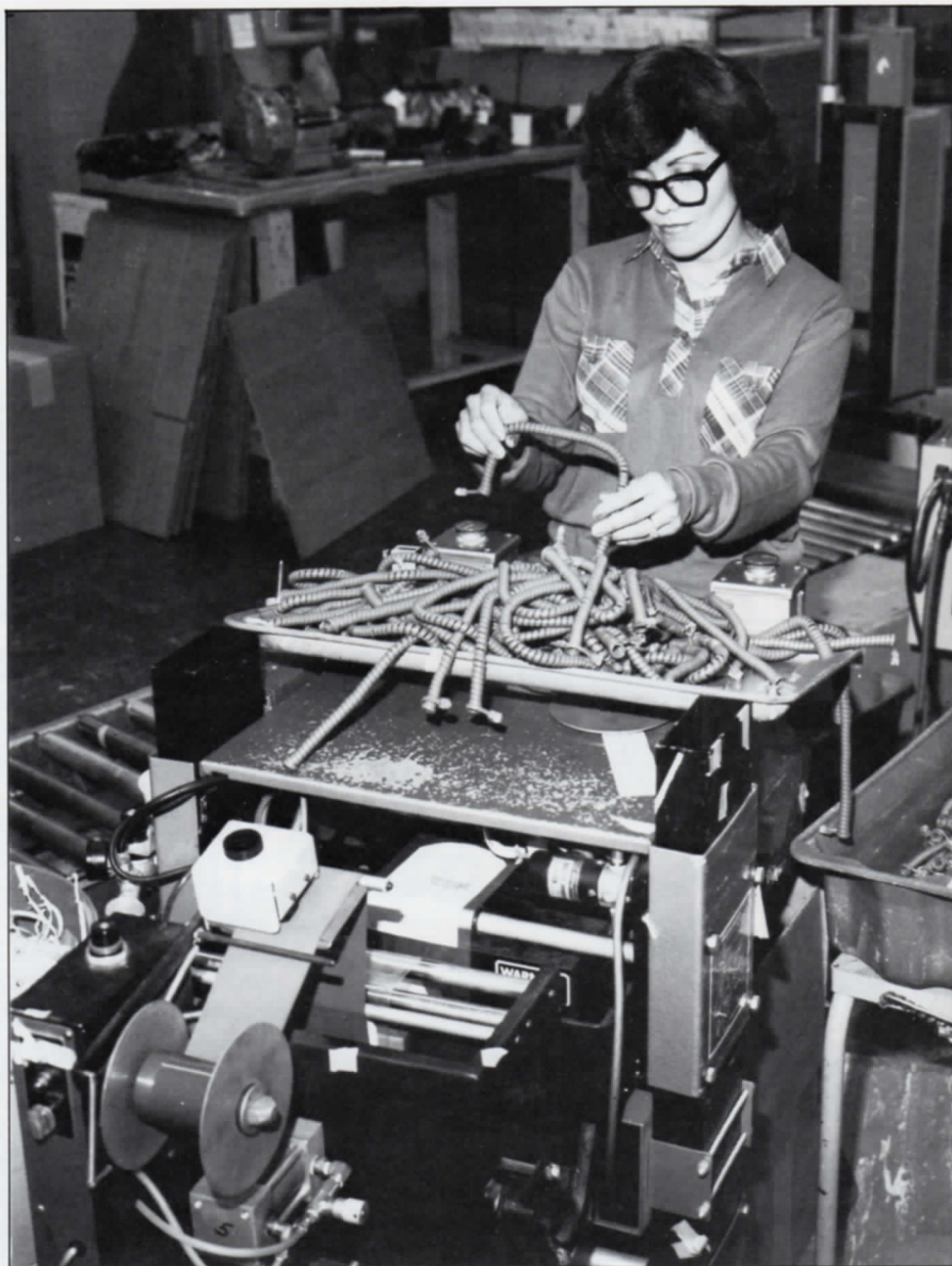
Preparing cords for bagging, Bea Gunia, 725, knows she works in safe conditions. The machine's electrical control system was modified to prevent accidental cycling during voltage surges.
