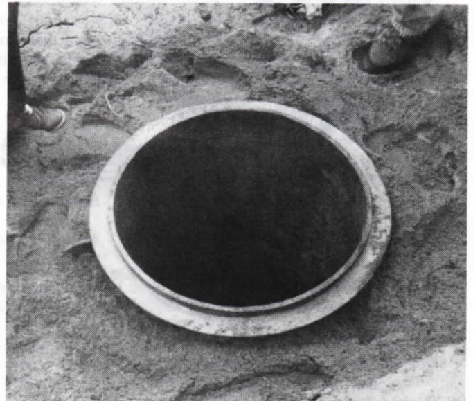
The launching tube is buried 8 feet into the ground.
