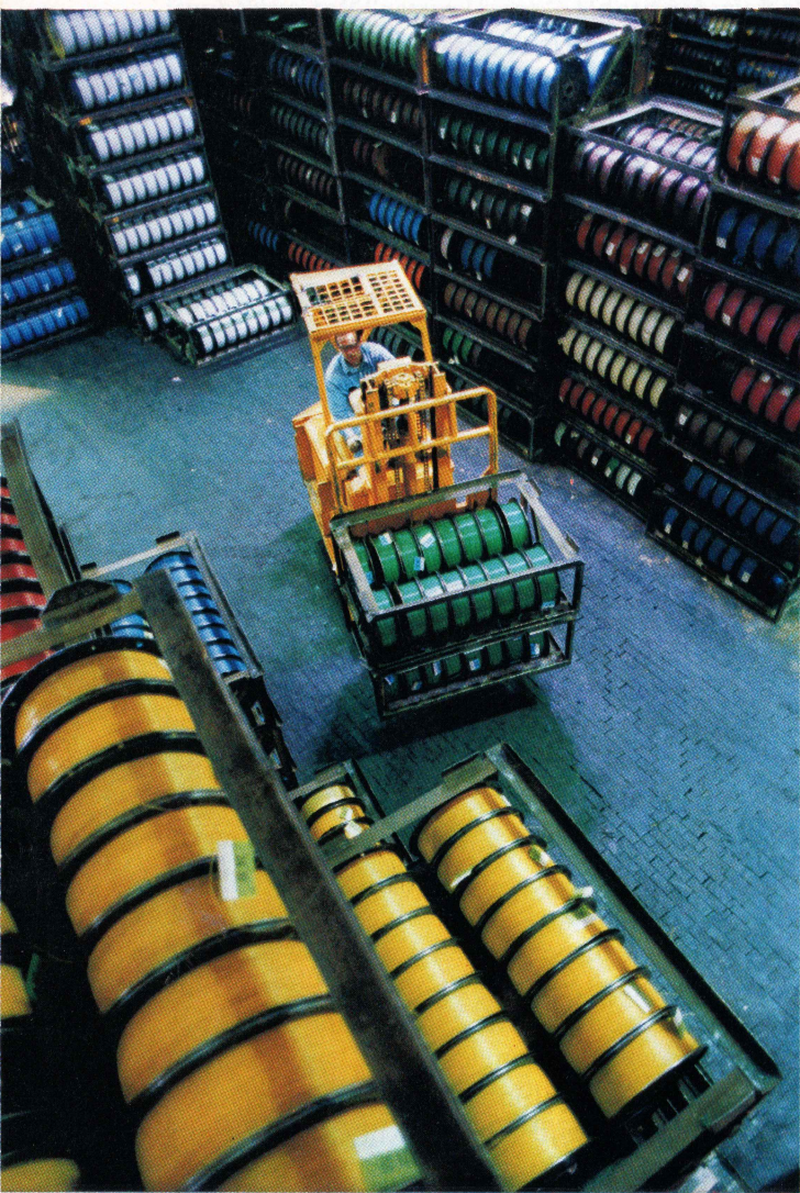
Above. At Omaha Works Norman Rohloff aligns wires, in this case 24-gauge polyethylene insulated, for feed into a cable strander.
