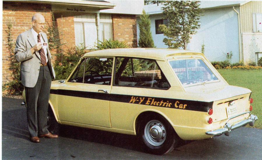
Paul Wergin of the Columbus Works and the W-Y electric car that he and fellow worker Dave Yates built. The unusual car runs on 16 six-volt batteries, has a range of 20 miles and costs about a penny a mile to run.
