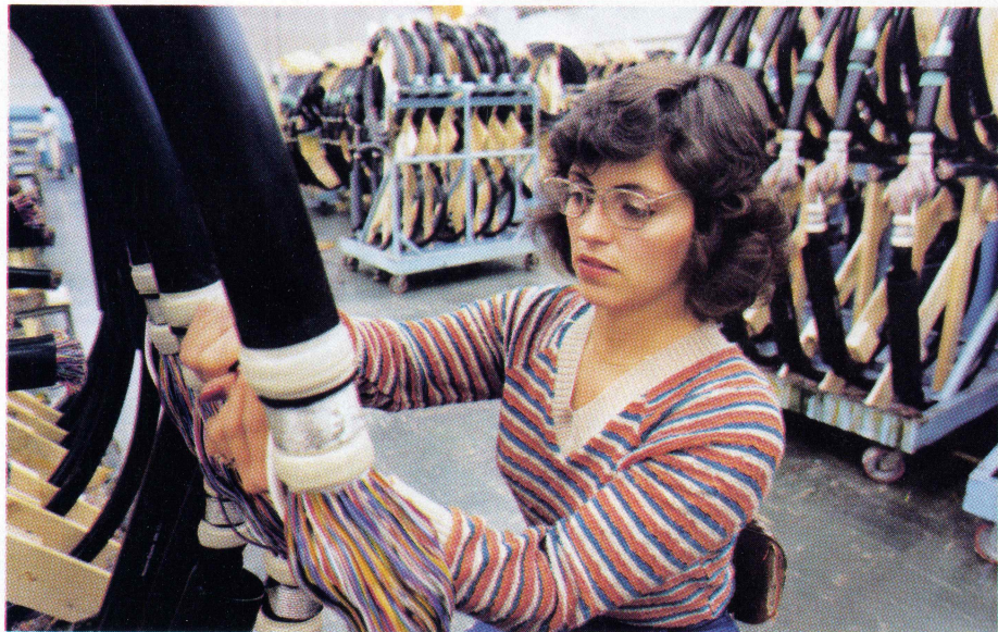
Above. Karen Moore removes binders from a 900-pair PIC cable stub, used to "stub out" some pairs for use outside the main pressurized cable run.
