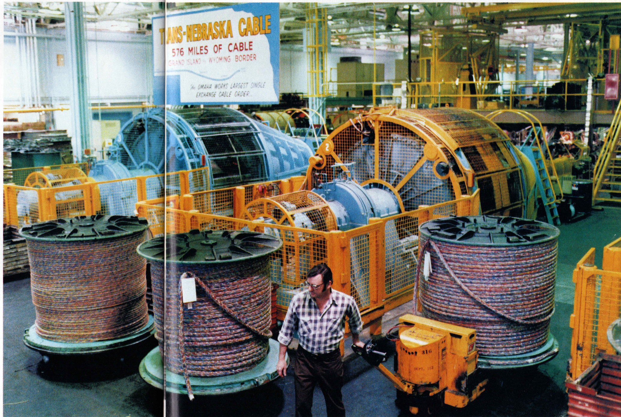
Above. At Omaha Works Norman Rohloff aligns wires, in this case 24-gauge polyethylene insulated, for feed into a cable strander.
