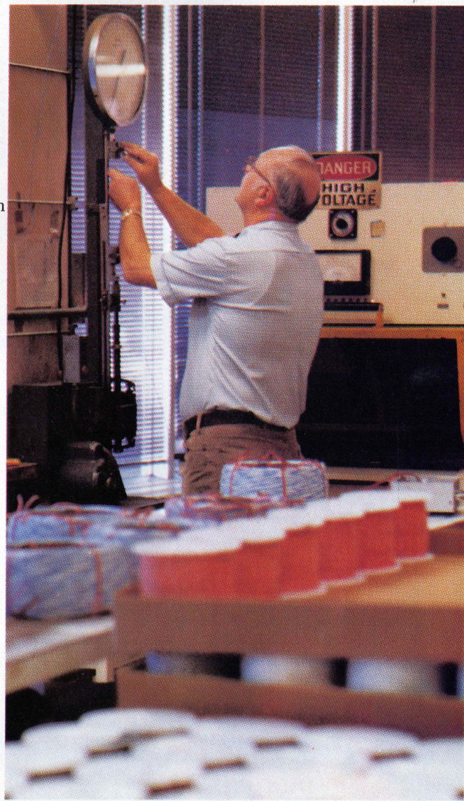
Above. Roy Schuster tests continuity and resistance of distributing frame wire prior to shipment. Right Bernice Salkeld adjusts a machine that braids tinned-copper wire around cable for electrical protection.
