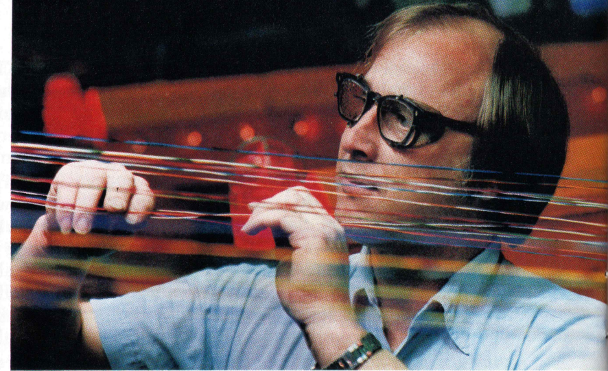
Above. At Omaha Works Norman Rohloff aligns wires, in this case 24-gauge polyethylene insulated, for feed into a cable strander.
