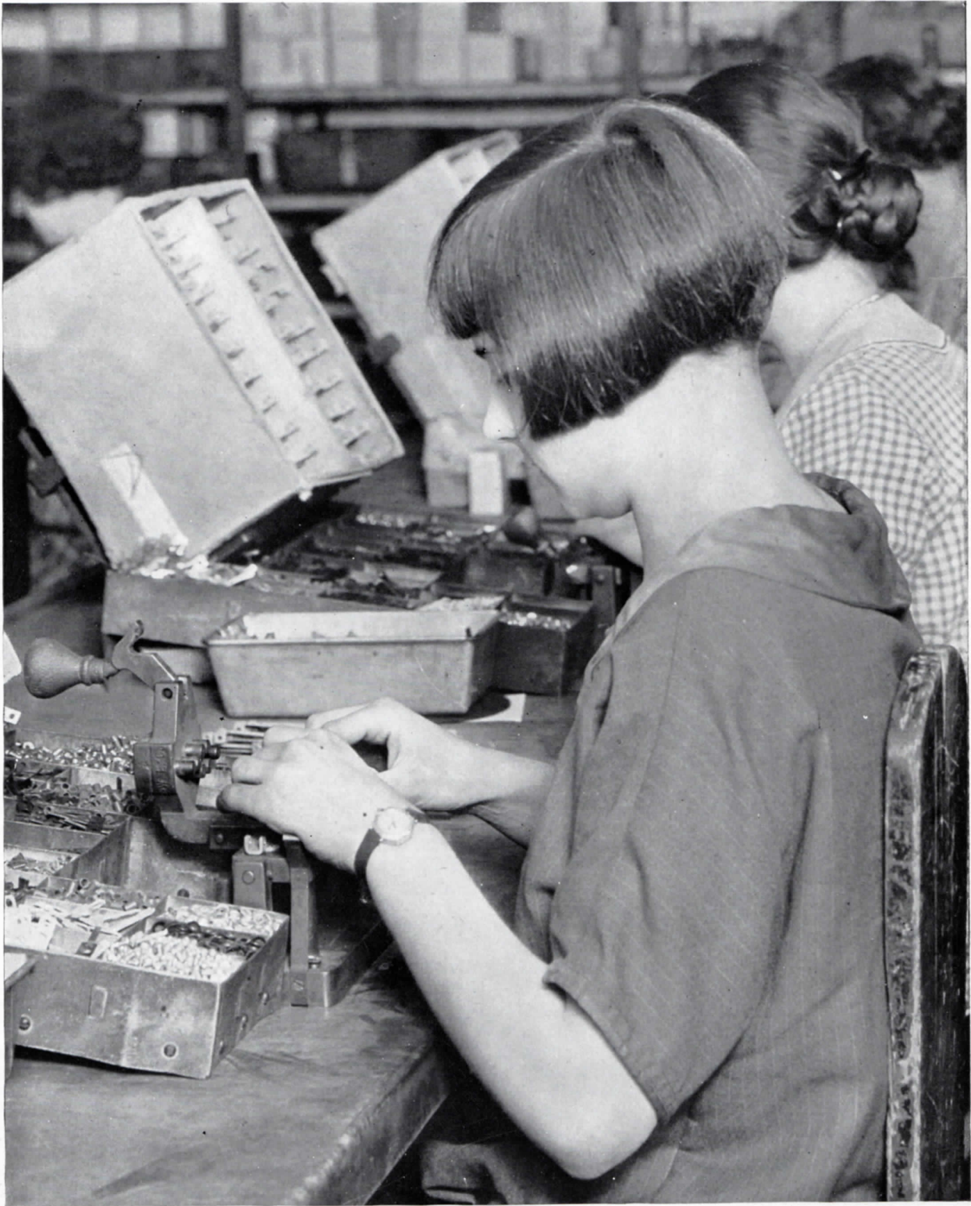
M ARIE TOMSCHIN, of Hawthorne, swiftly assembles terminal plates for desk stands, but speed is not allowed to interfere with accuracy
