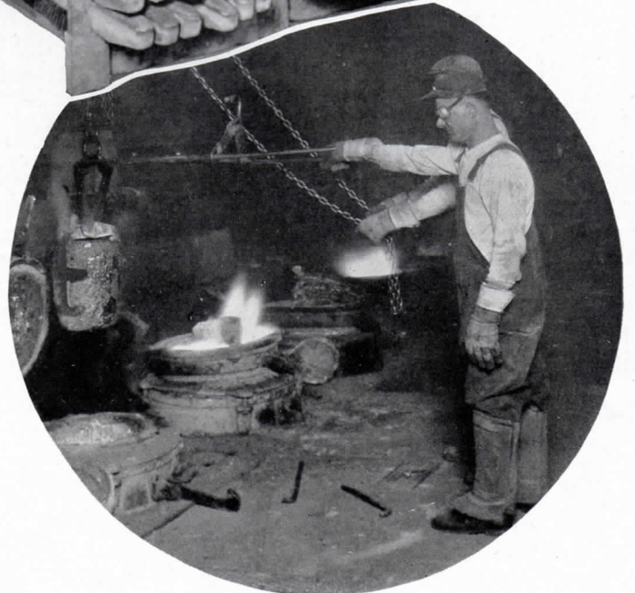
A row of roaring kettles, in which the soup consists of various copper, aluminum, zinc, and other non-ferrous metal alloys. A crucible with a melted metal mixture ready for pouring is being lifted from the fire by means of a manually operated hoist
