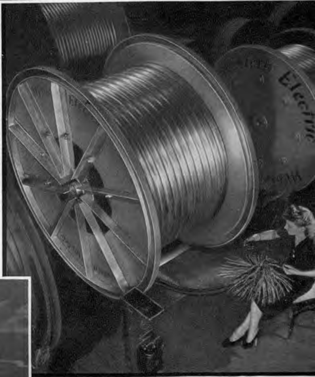
Keeping careful watch while stranding telephone cable.
