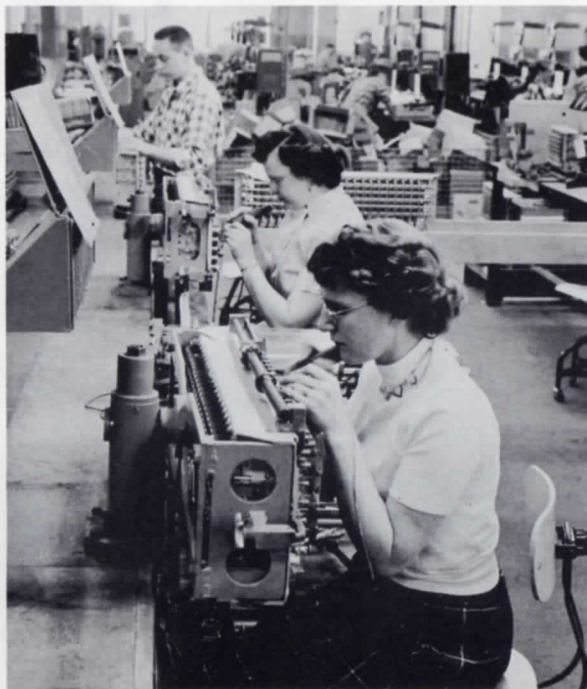
Phyllis Ocander and Betty Chesnut solder connections of terminal ends of springs in the horizontal strapping operation, one of some 30 manufacturing and testing jobs performed before an intricate crossbar switch is fully assembled and ready for shipment.
