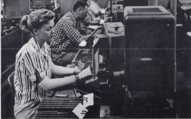
More than 2.8 million precious metal contacts are welded to wire spring assemblies each week. Shown above are some of the men and women, and machines, responsible for this big job. They are, front to rear, Darlene Schriefer, Paul Hosch, Aletha Ferguson and Juanita Bailey.
