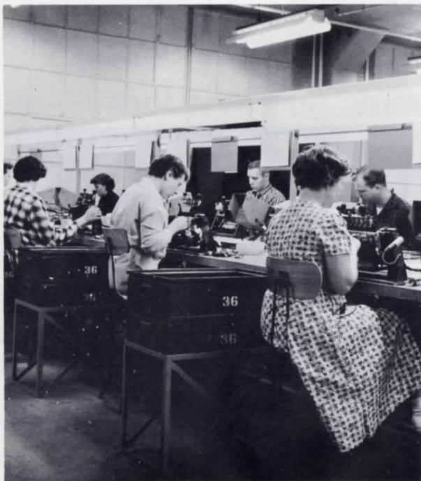
Adjusting and inspecting vertical units for the crossbar switch are, left to right, Rosalie Ross, Cecilia Wilcox, Gwen Zimmerman, inspector Rodney Olson, Hertha Bishop and Fred Herre. The crossbar switch is a principal switching element in modern telephone dial equipment.
