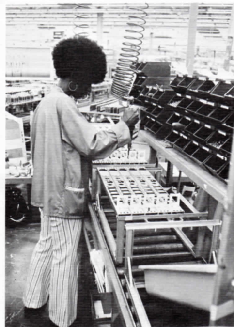
If the WSR stays in-plant for use in a Crossbar frame, for instance, the relays are mounted in mounting plates and stamped to facilitate identification in the field, as illustrated by Esther Curry (above).
