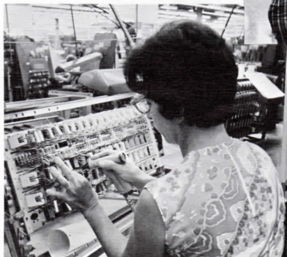
If the WSR stays in-plant for use in a Crossbar frame, for instance, the relays are mounted in mounting plates and stamped to facilitate identification in the field, as illustrated by Esther Curry (above).
