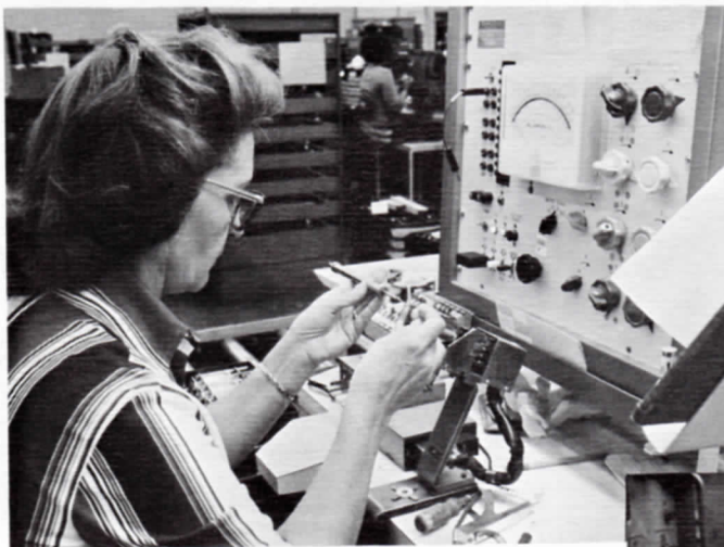
Elaine Peterson (above) and other Relay Adjusters "fine tune" the assembled relay to insure that it will function according to expectation when it goes to work.
