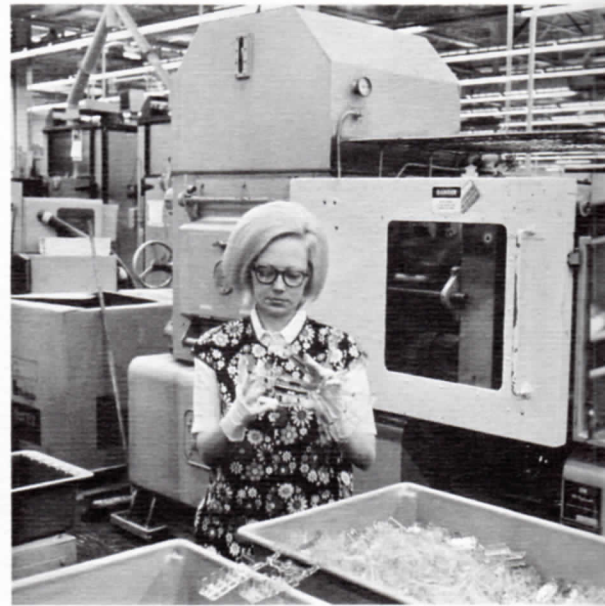
Molding dust covers -- 12 at a time -- is the job of Bea Klaumann. She runs two injection molding presses at the same time.
