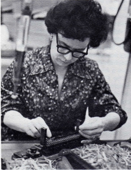
ROW BY ROW . . . Beverly Prather assembles the mounting strips, swiftly and smoothly placing the terminals in rows on each strip.
