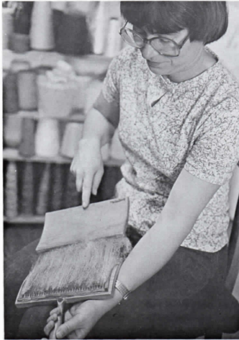
FLUFFY . . . Mary Jo Horning first fluffs up wool by pulling it between two wire brushes (left), a process called "carding." Then a few fibers of wool are wrapped around a leader piece of yarn, which is threaded through the flyer and onto the bobbin. She holds the fluffed up wool as the flyer twists it (right).
