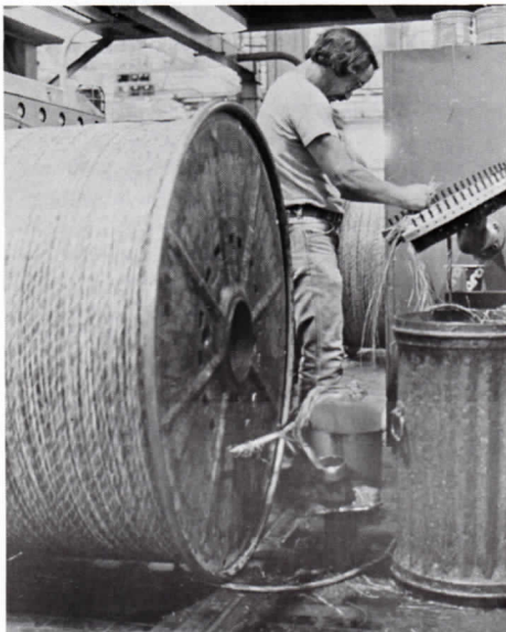
TESTING . . . Rock Ferrucci of Dept. 252 checks the electrical capabilities of cable core on a full reel. Rock also operates a flyer stander in his department.
