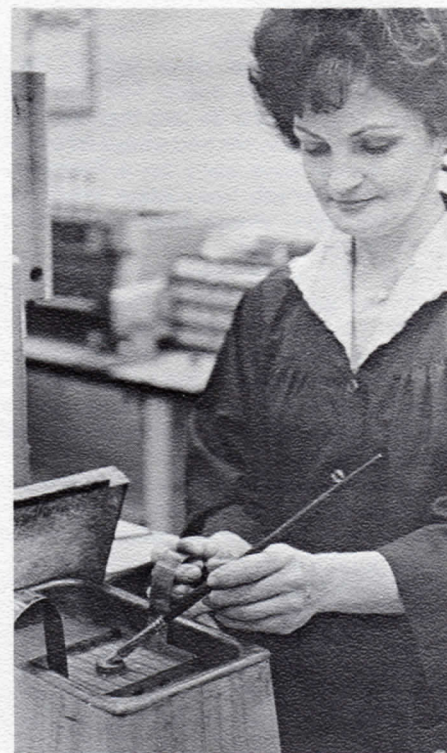
CLEAN WAVE . . . Sue Ellis cleans a die in an ultrasonic solution, part of the process involved in reshaping dies on an ultrasonic die processing machine.
