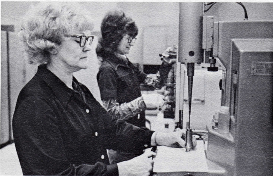
TEAMWORK . . . Jane Phillips (foreground) reshapes a fine gauge die ultrasonically, while Judy DeVault polishes fine gauge dies on a wire lapper.
