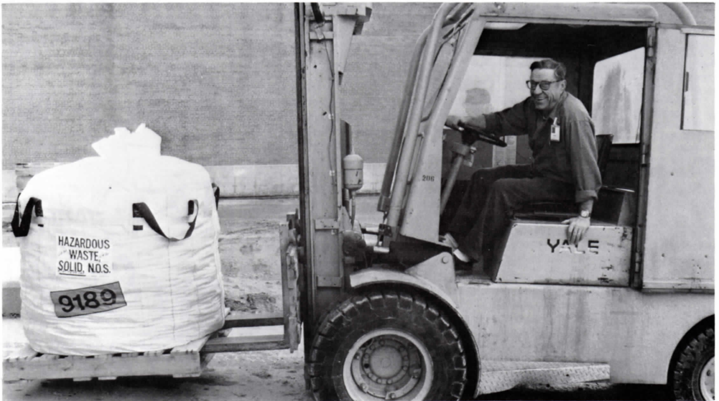
IT'S IN THE BAG . . . Waste treatment plant operator Glenn Lund, Dept. 558, moves a bag of solid waste — metals precipitated from waste water — to the outside of the plant to await disposal at a landfill. Waste treatment produces about one 1800-pound bag of the modeling clay-like waste each day.
