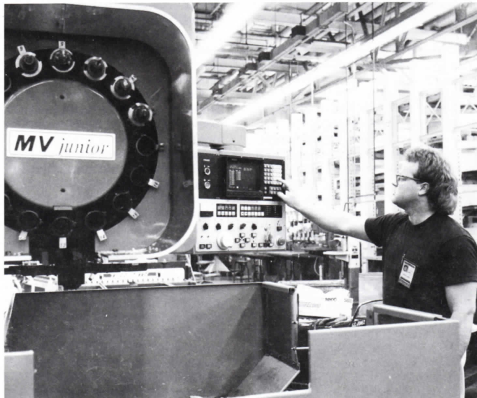
AT THE CONTROLS... Operating the Mori Seiki CNC (computer numerical controlled) milling machine is only one part of the job for Dwayne Hanel in the custom fabrication shop.
