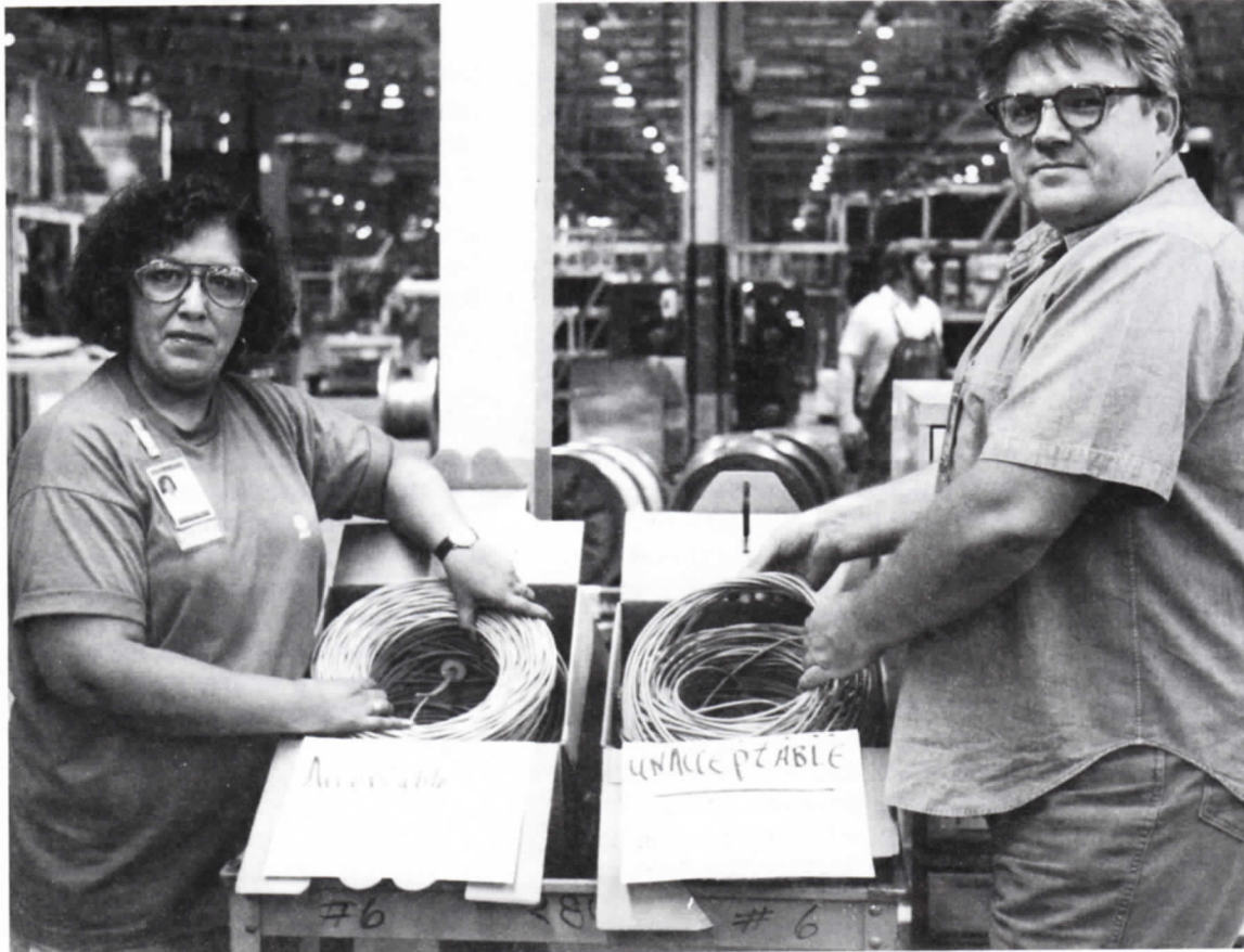
SEE THE QUALITY... Pam Moreno grips properly coiled wire and it keeps its shape. When Ron Schmidt grabs hold of an unacceptable wire coil, it pulls apart, a sign that it will tangle when used by an installer.
