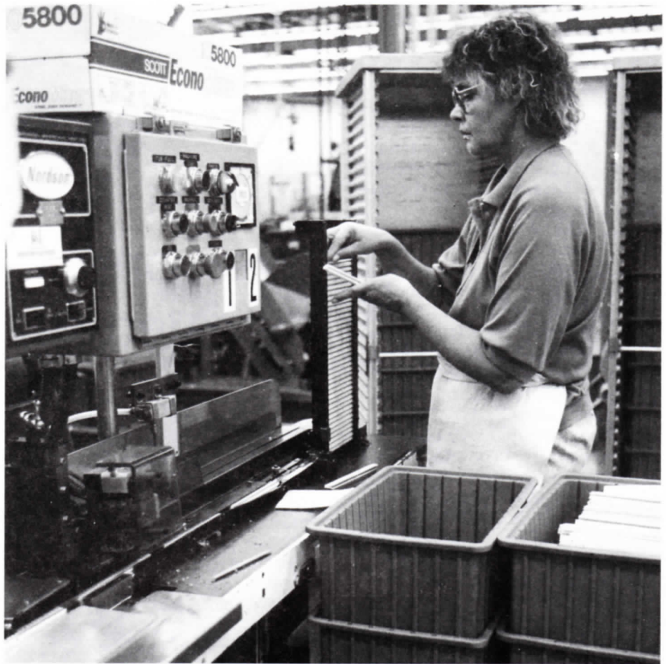
THE RIGHT AMOUNT...Production employee Mona Johnson operates the "fill and bag" machine used to fill 710 connectors with waterproofing encapsulant prior to automatic bagging. As she loads connectors onto the machine, she watches for missing terminals, too.
