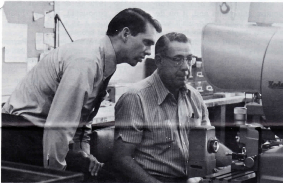
Curt, left, and Vern use a Kodak Comparator to determine if a piece parts meets specifications.
