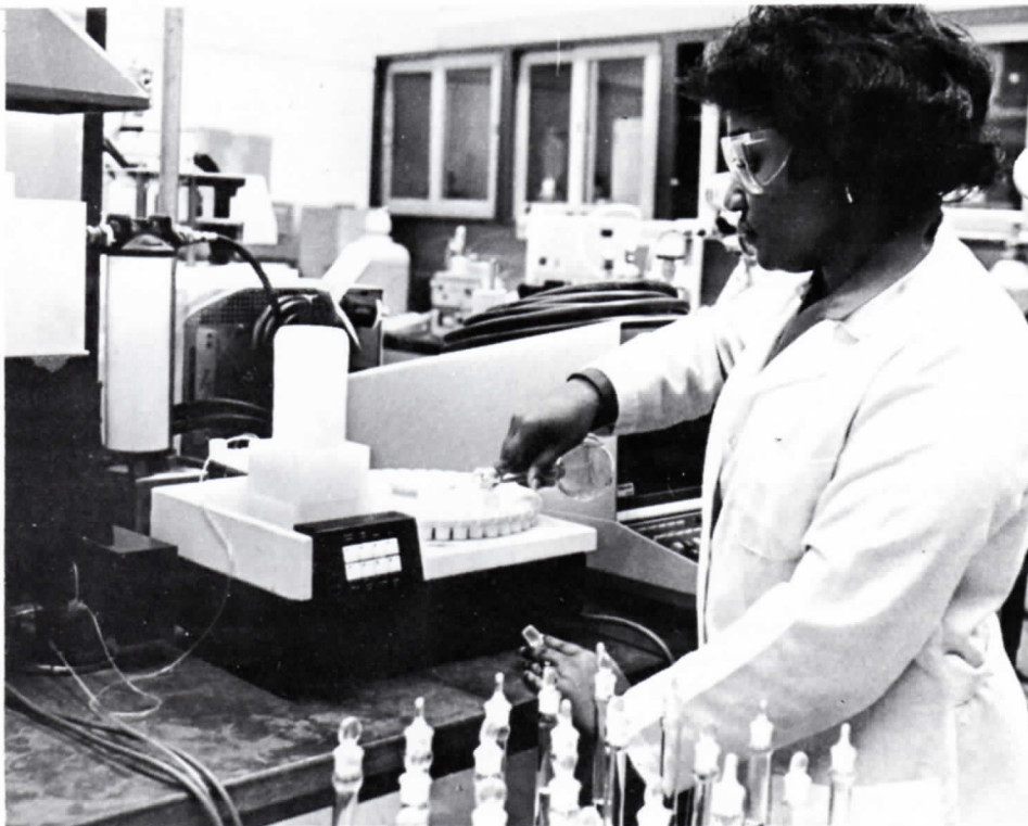
IS IT GOLD? . . . Loretta Lewis relies on a direct current plasma spectrophotometer to help her determine the gold content of a solution she pours into a test tube.
