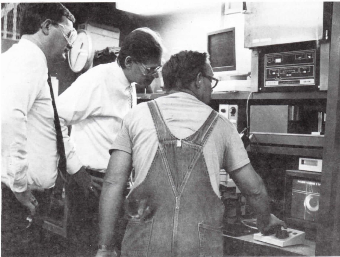
HOW THICK IS IT?... IBU 559 insulating line operator Ron Nelson (right) demonstrates to Anixter's Pete Lockhart (left) and Mike Hecklinski how computer testing is done to determine precise wall thickness of insulation on wire for local area network (LAN) cable.
