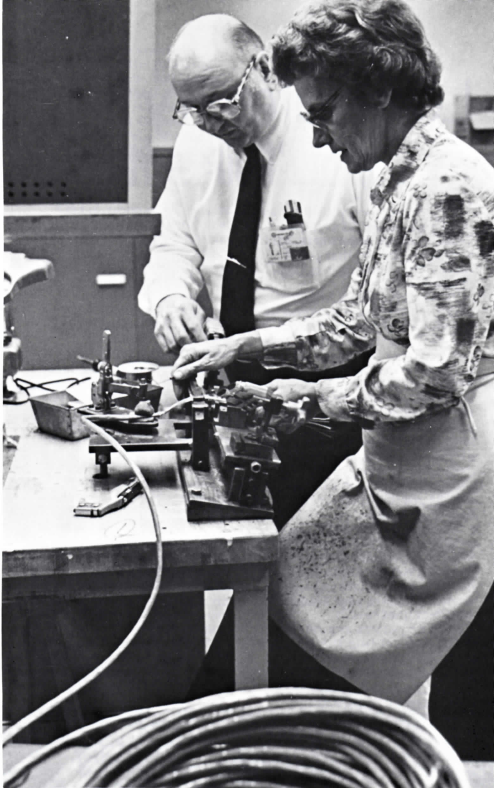
TAKE IT OFF . . . Assembler Marlys Schoville of Dept. 287 strips insulation from the conductors of Olympic cable in preparation for connectorization. With her is engineer Walt Onisk.
