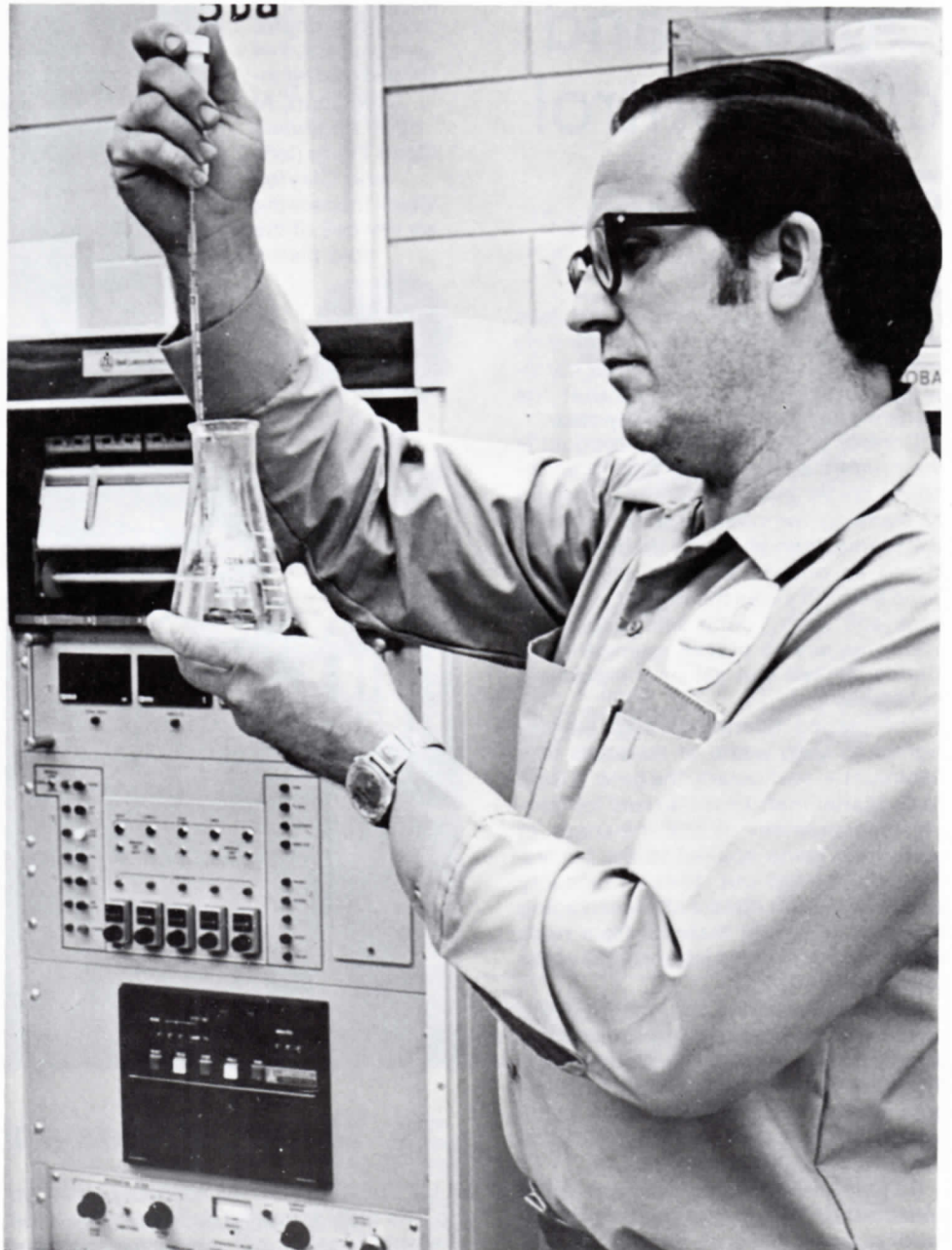
HOW RICH IT IS . . . Layout operator Larry Griff samples the gold plating solution which will be analyzed to determine how many grams of gold are present.
