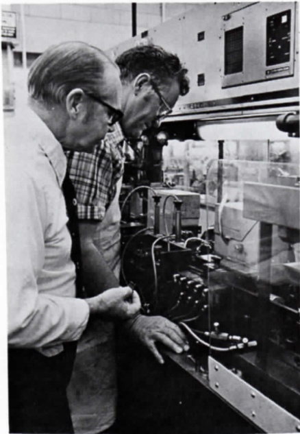
SAFETY PRACTICED . . . Bob Morey (left) and Jerry Proctor watch the operation of an in-line welder, one of the machines in Dept. 728 featuring guards (visible in foreground).
