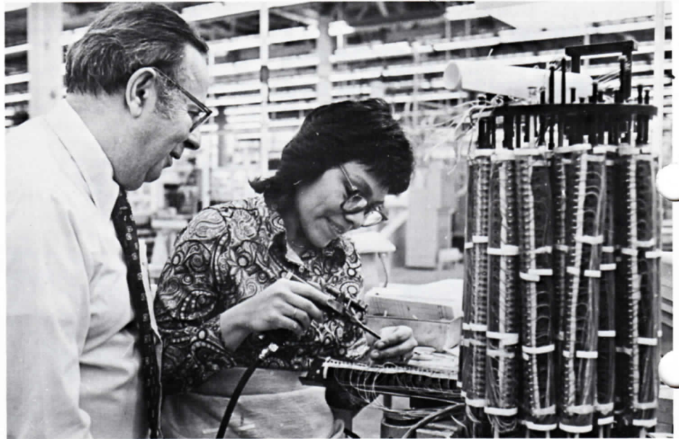
INS AND OUTS . . . Victoria Balsarini is one of the people in Dept. 444 who helps make sure Mike Szymanski's "baby" flies. She's wiring the "in" and "out" wires of cable to a 600-coil load coil before it is encased in a polyethylene cover.
