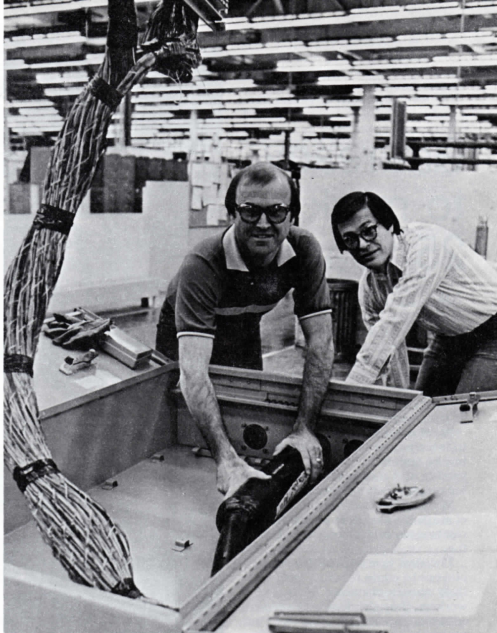
FOR IRISH EYES . . . The packing team of Jim McDonald (left) and Joe Backes of Dept. 439 were responsible for packing the two 40-type cabinets for Ireland. Before packing them in wooden boxes, they made sure the stub cable was secured and they installed the wired frame into each cabinet.
