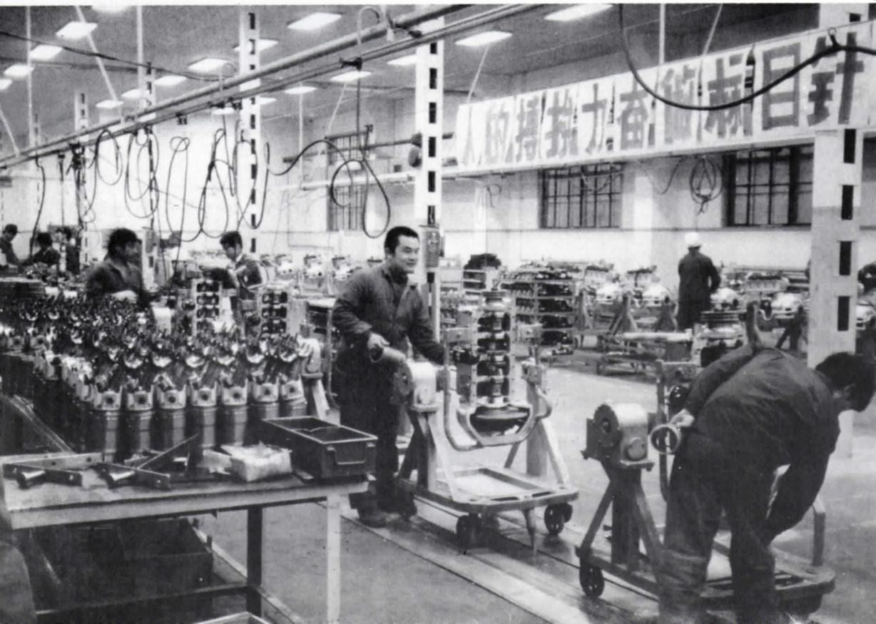
ASSEMBLY LINE ... A factory worker mounts pistons in the block of a truck engine at a plant in Beijing. A productivity slogan hanging in the background states, "The human struggle will achieve the goal."
