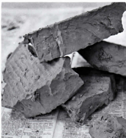
PIECE OF CAKE . . . A new filter press transforms plant sludge into the consistency of yeast cakes. So long, pea soup.
