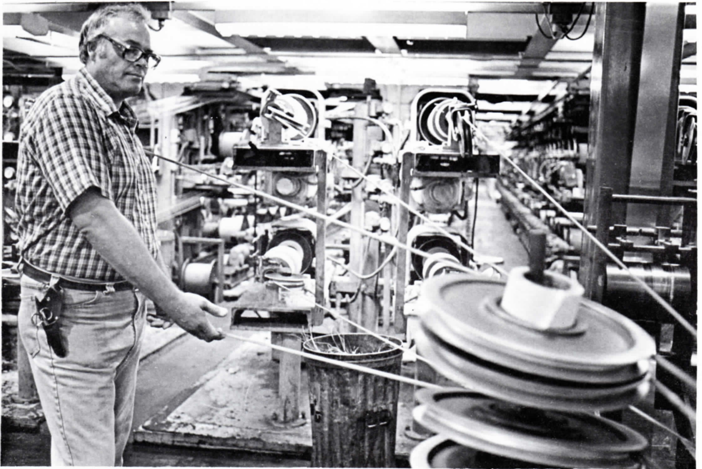
SMOOTH RUNNING . . . After 20 years of service in the cable shop, Mike Lewts of Dept. 252 knows his job well. A layout operator, he's checking the base plate of a stranding machine to make sure wire is feeding into it properly in the manufacture of Z-screen cable.
