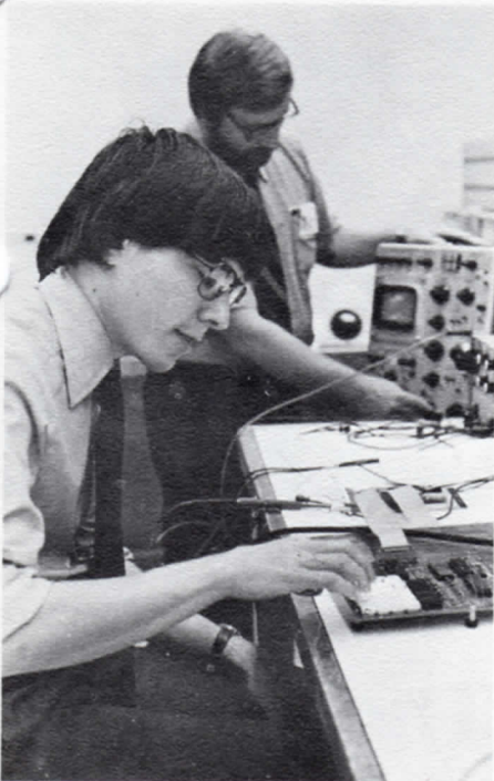
LAB WORK . . . Gilles Heyart and Steve Zerbs (back) use a microprocessor kit to simulate insulating line capacitance measurement.
