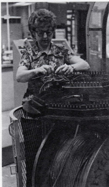
CABLE CHECK . . . Judy Thoms of Dept. 1231 prepares to test R-switchboard cable (irradiated) using a high-voltage dielectric strength test set.
