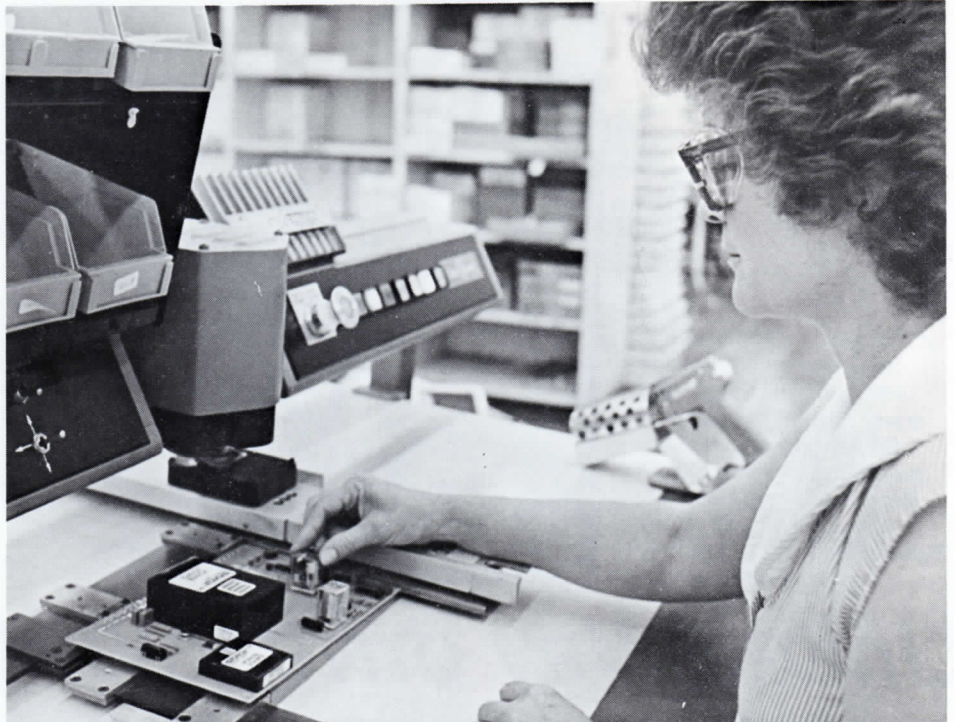
CIRCUITRY . . . Mary Nowak of Dept. 441 operates a machine used to assemble a circuit board for the 190A test set. The machine automatically provides the correct part and indicates where it is to be inserted.
